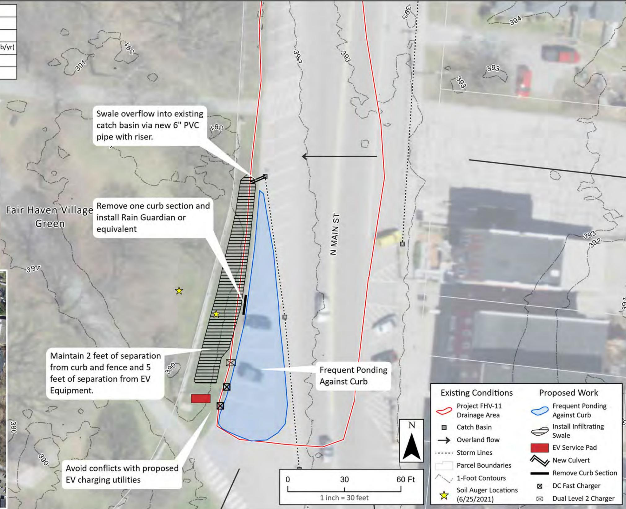
Swale overflow into existing catch basin via new 6" PVC pipe with riser.
