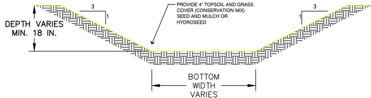
**Detail B: Sediment Forebay and Infiltration Basin**
